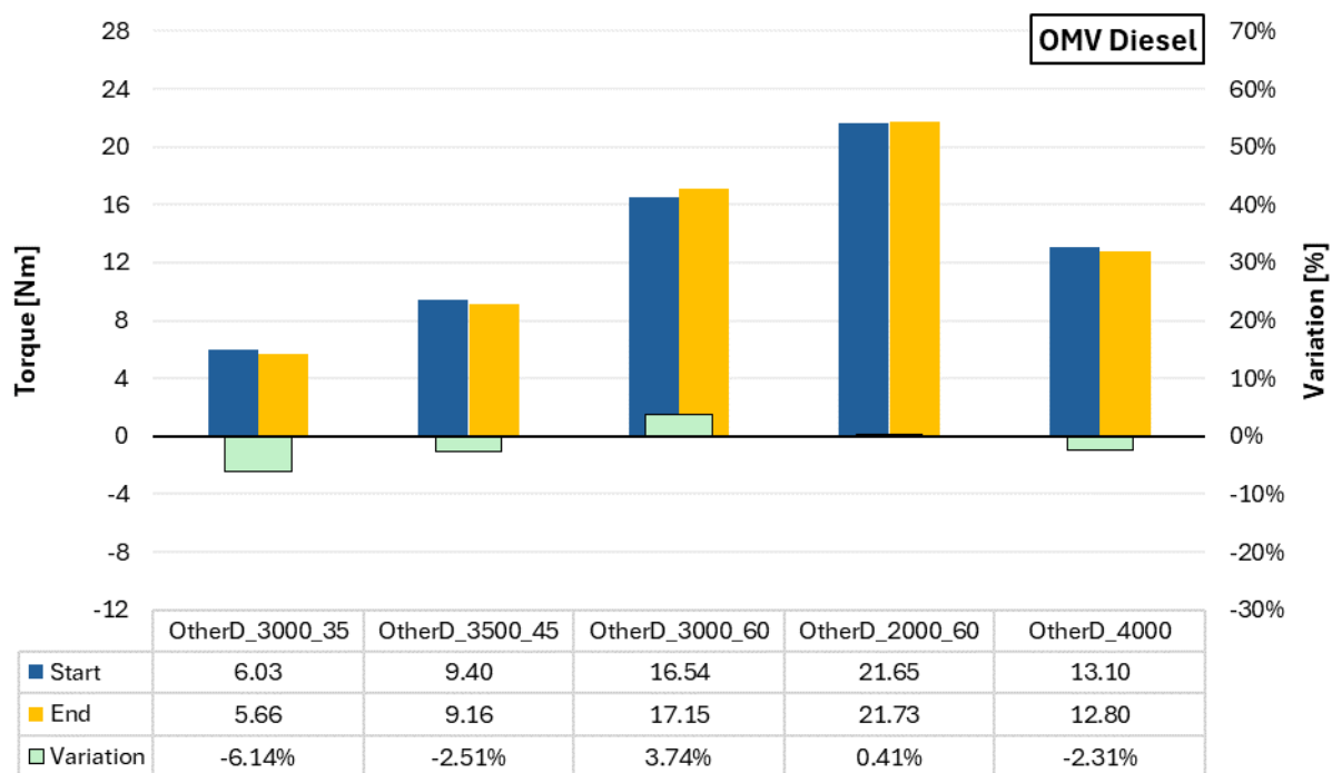
Fig. 4.8 OMV Diesel – 32 h Start-End torque variation
